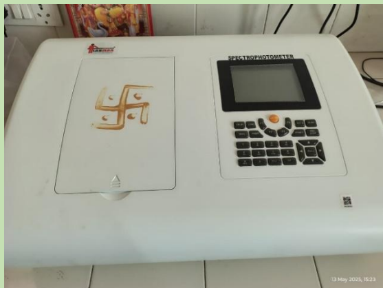
UV Visible Spectrophotometer (LABMAN Double Beam UV-Vis. Spectrophotometer - LMSPUV1920)
